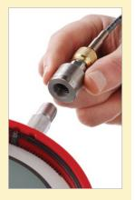
Connect these adapters with female Ralston Quick-test™ ends directly to a Ralston hand pump, volume controller, nitrogen source or calibration manifold. The user can switch NPT sizes depending on the process connection of the gauge they are calibrating.
